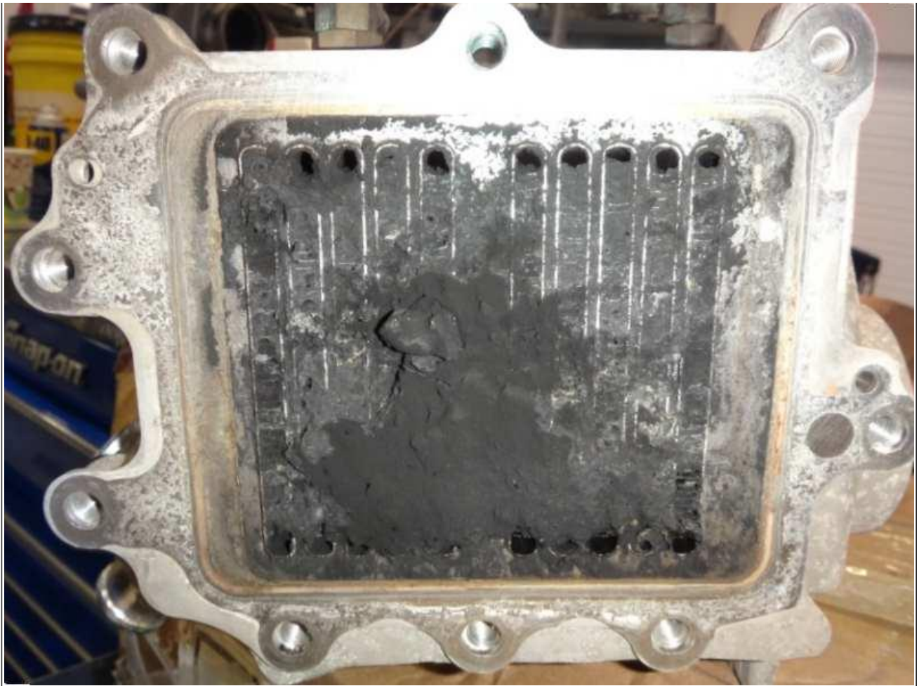
Figure 12: Soot Build-Up on the Core Face
