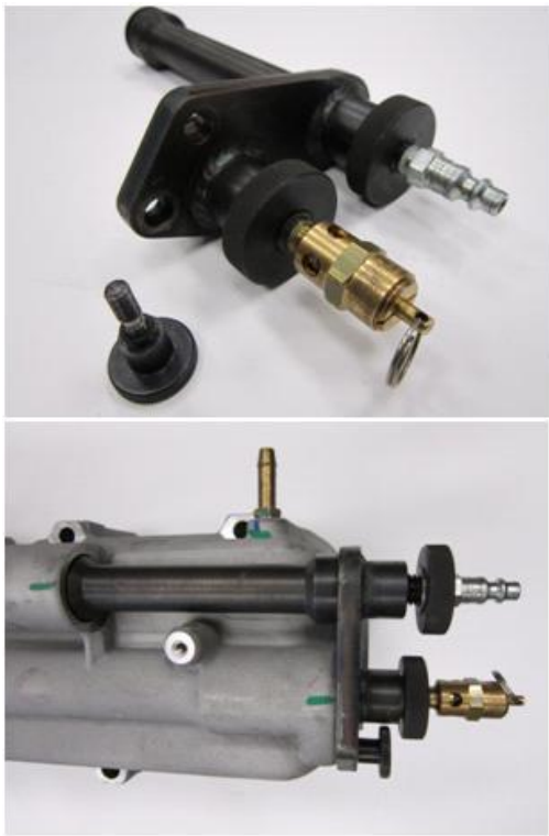
Figure 4: Coolant Port Plug
