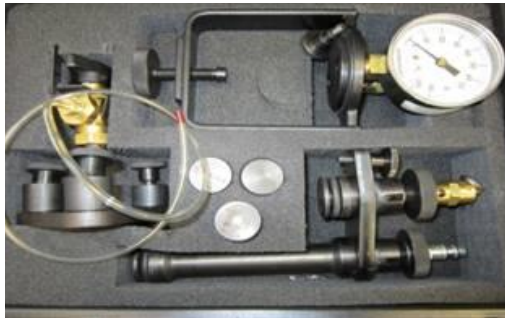
Figure 2: KL20030NAV - EGR Cooler Leak Detection Kit
