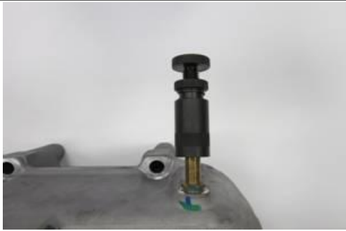
Figure 3: Deaeration Fitting Plug
