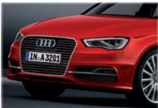
e-tron specific front bumper with two aluminum-look surrounds on the air intake covers
