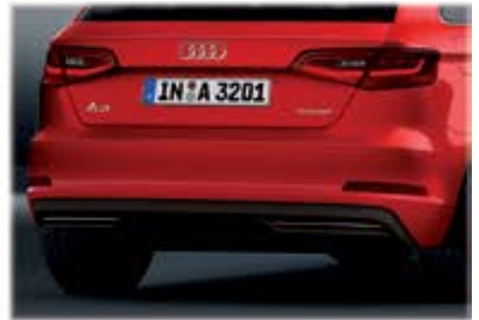
e-tron specific rear bumper with diffuser, aluminum-look surrounds and concealed exhaust pipes
