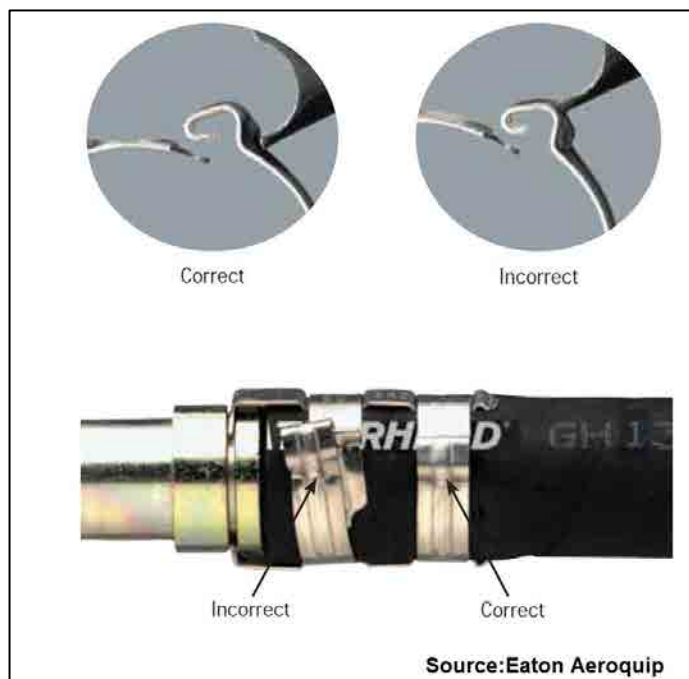
Figure 13 : Clamp ring clasp recommendations
