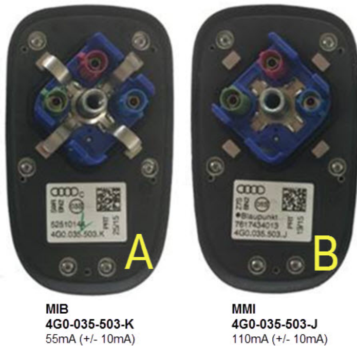
Figure 5. MIB antenna with K suffix part number 4G0-035-503-K (A), and MMI antenna with J suffix part number 4G0-035-503-J (B).
