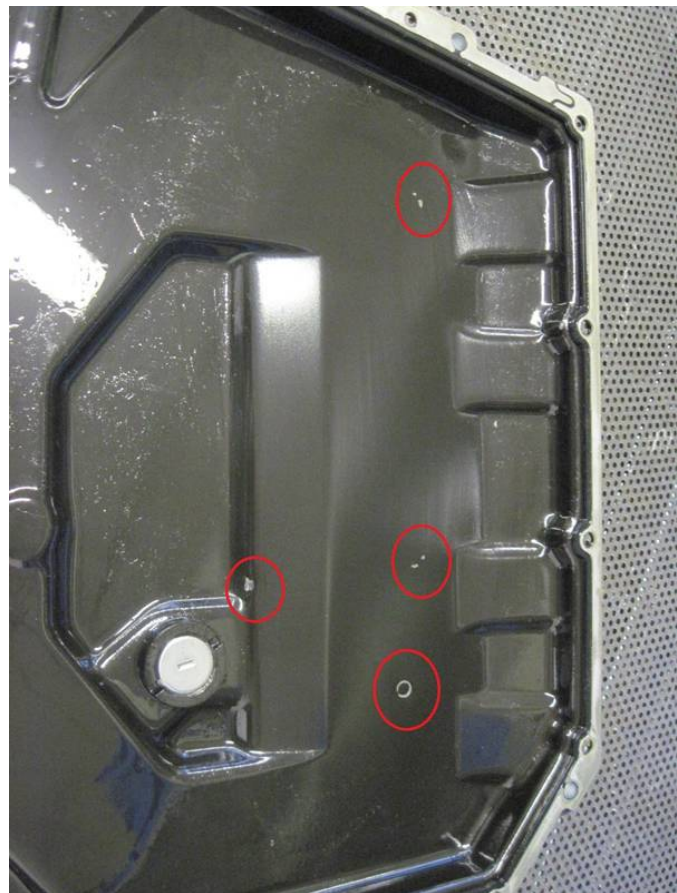
Figure 5. Damaged oil sump because of loose bolts.
