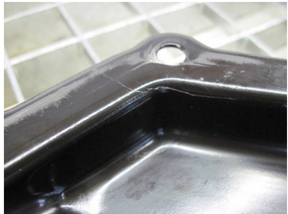
Figure 2. Crack in the oil pan.
