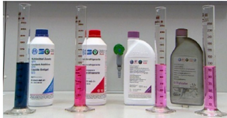
Figure 1. The color of each type of engine coolant. G11 (green-blue), G12 (red), G12+, G12++ and G13 (purple).
