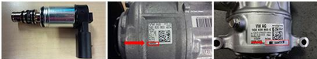
Figure 1. N280 Refrigerant Regulating Valve. Figure 2. Denso compressor identification tag. Figure 3. Sanden compressor identification tag.
