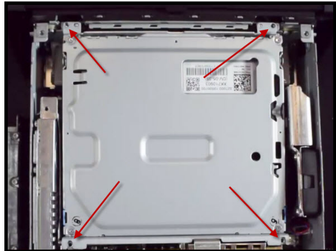
Figure 11. CD drive mounting points are now free.
