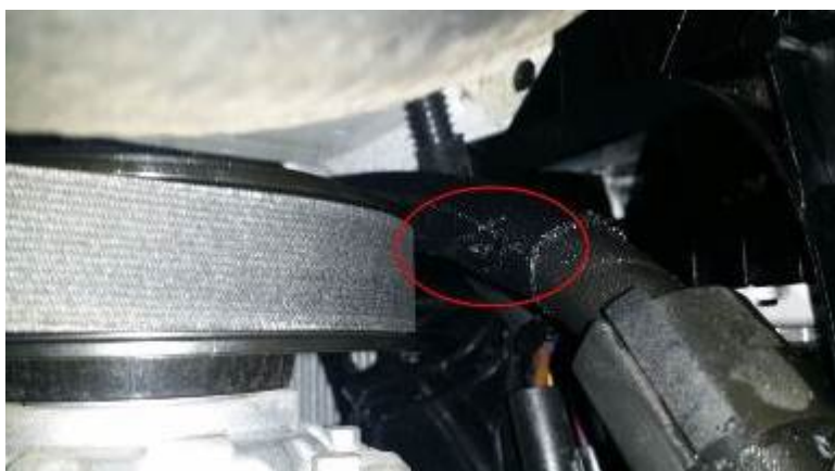
Figure 1. Point of hose contact with air conditioning compressor pulley.
