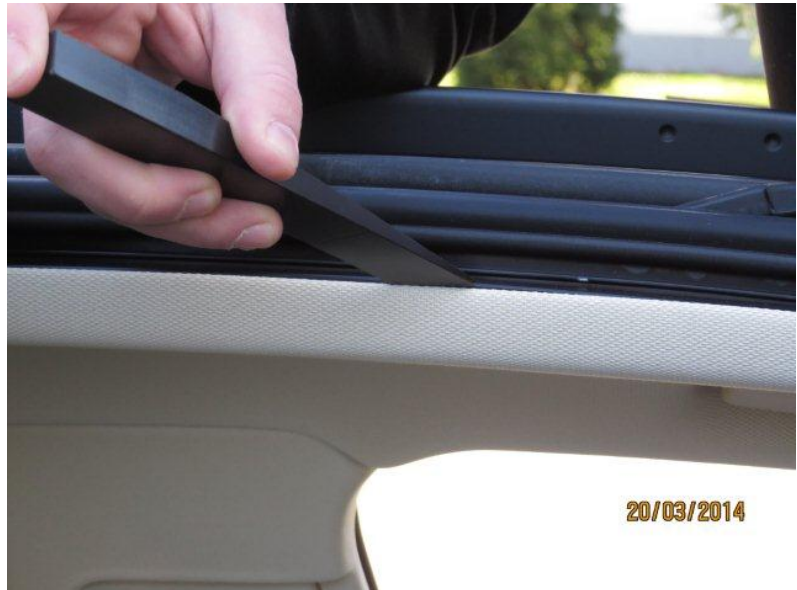
Figure 1: Unclipping the sunroof cover trim frame.
