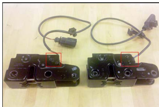
Figure 3. The mounting locations for the contact switches 8T0953236B and 8K0953236A are different; thus, they are not cross compatible.
