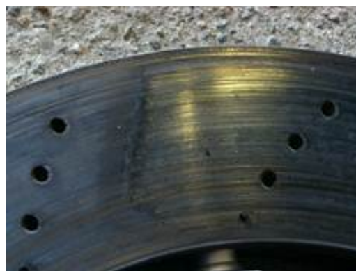
Figure 2. Deposits on the brake disc.
