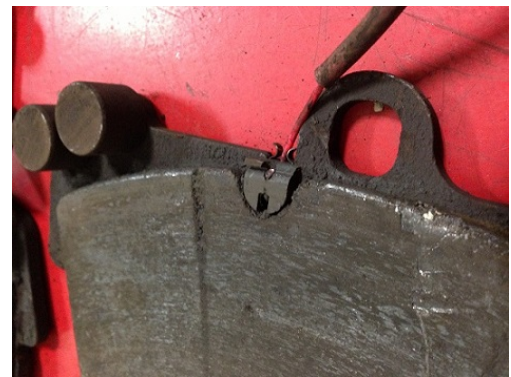
Figure 7. Worn brake pad.
