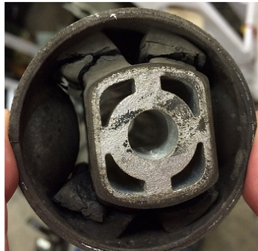
Figure 8. Damaged suspension bushing.
