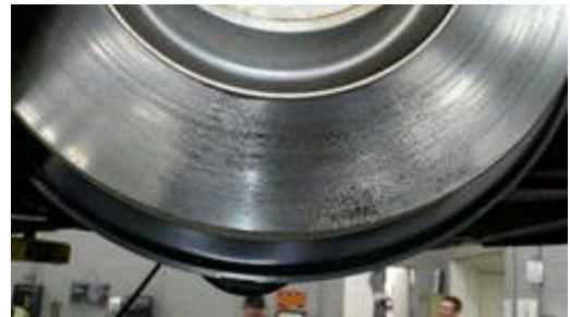
Figure 5. Pad marks on the brake disc.
