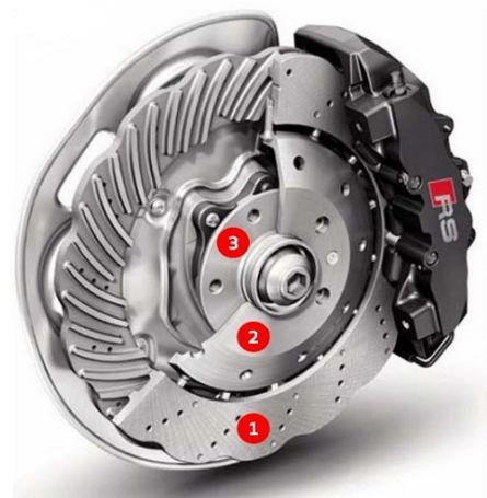
Figure 12. Run-out measurement locations: disc braking surface (1), disc hub (2), wheel hub (3).
