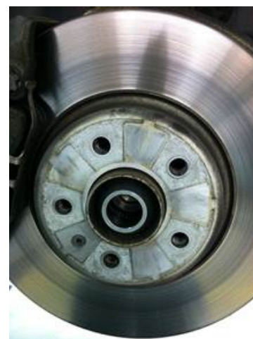
Figure 3: Brake disc with heat marks.
