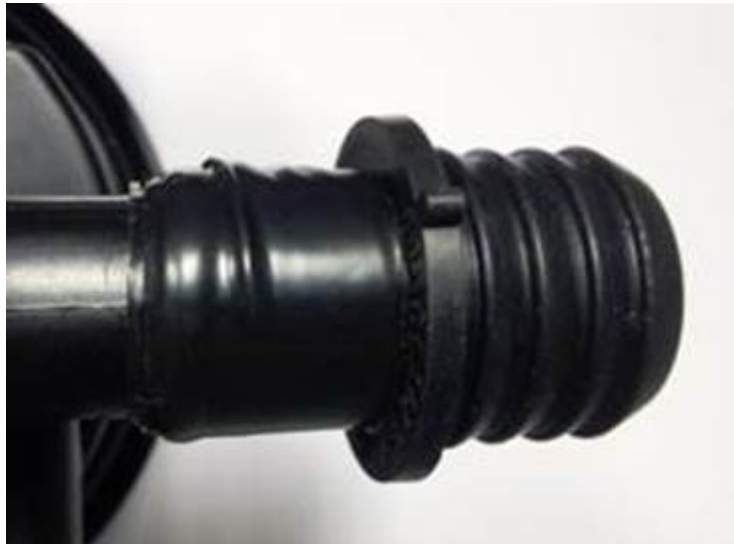
Figure 4. Vinyl layer supporting grommet.
