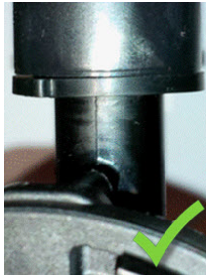
Figure 6. Correctly-installed sensor and grommet.
