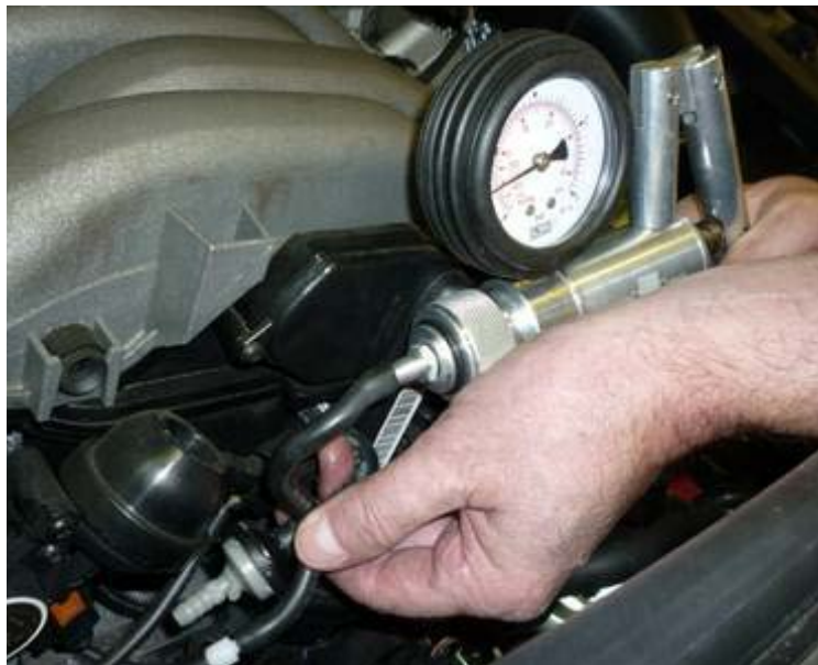
Figure 2. VAS 6213 hand vacuum pump
