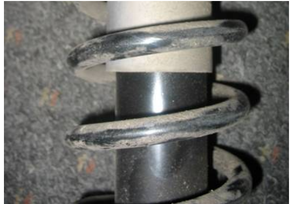
Figure 3. A shock absorber that is not leaking.
