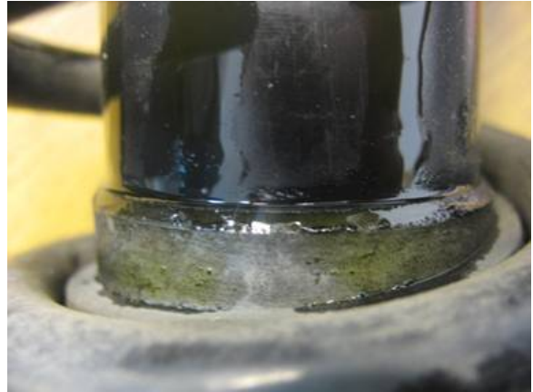
Figure 1. A leaking shock absorber.
