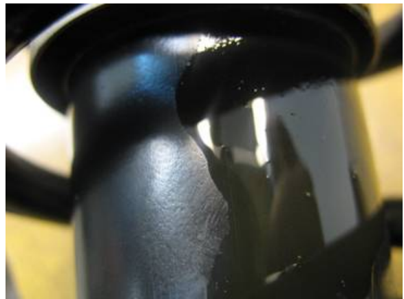
Figure 2. A leaking shock absorber.
