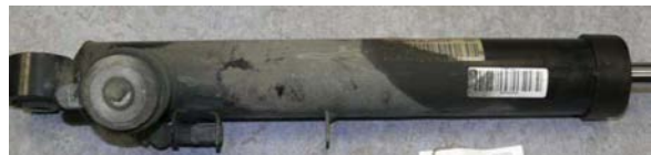
Figure 4. A shock absorber that is not leaking.
