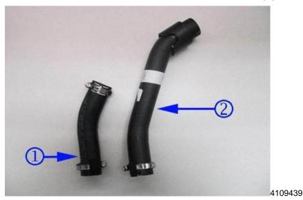
2. Match the new hose (2) to the original (1), aligning side by side.
