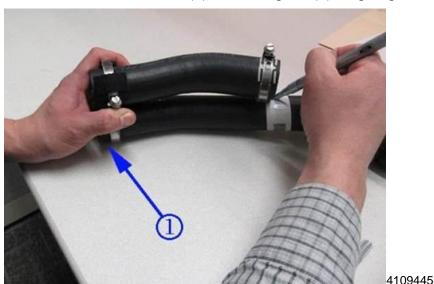
3. Using a paint pen or equivalent, mark the new hose to the original, starting with the notched fuel tank ends of the hoses so that both hoses are the same length.
