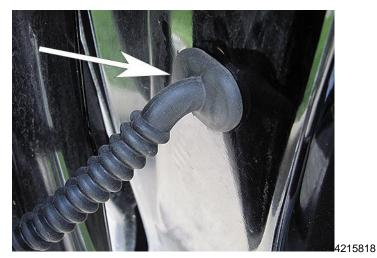
2. Remove the rubber boot from the door pillar. Gently pull the body harness through the hole exposing the connectors.
