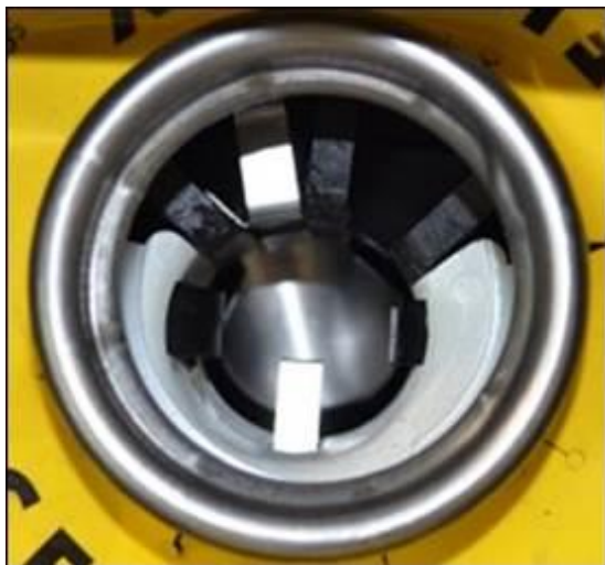
Figure 1. Misfueling guard installed in the filler neck.
