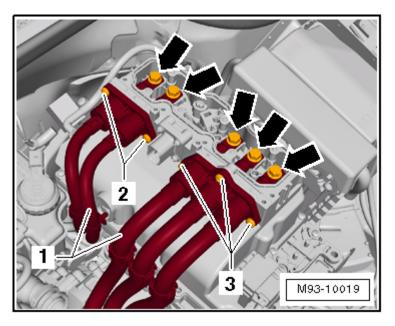
Tightening Specifications, High Voltage Contacts
