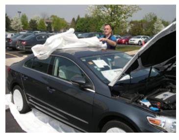
• Cut the upper FBC around the windshield and roll cover towards rear of vehicle.
