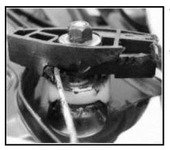
Window regulator cable retainer is broken. The material of the retaining clip (POM) is too hard.
