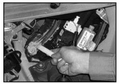
• Apply polyurea based grease (obtained locally) to front and back of guide rails (A, B and C above) and cursers using wedge tool Part No: 3409.
