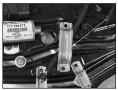
• Pass the cables through carrier plate support brace (as required).
