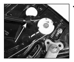
Route upper cable around upper pulley and seat upper cable guide into slot -arrow-.
