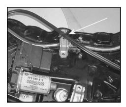
• Free window cables by cutting the tie strap -arrow- at upper carrier plate support.
