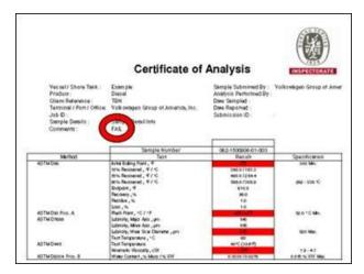
**Figure 11.** Example of a contaminated fuel analysis.
