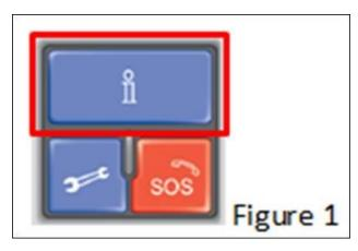
First attempt to verify the customer complaint by pressing the "i" button (see Figure 1) in the overhead console.
