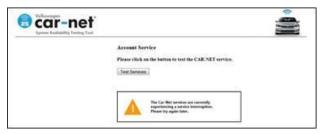
If the result shown after clicking the "Test Services" button indicates that the Car-Net Verizon Telematics system is experiencing a service outage or interruption, no further diagnosis of the vehicle is required. The customer complaint is the result of the service outage or interruption.
