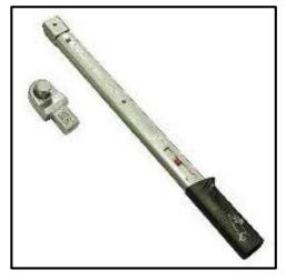
VAG1332 – 40-200Nm Torque wrench (or equivalent)
