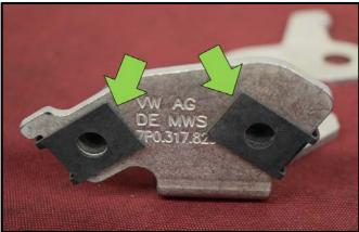
Affix the speed nuts, P/N: N90168604 onto the bracket, P/N: 7P0317829 as shown <arrows>.
