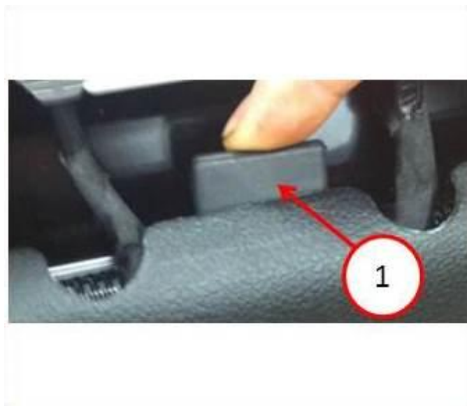
Fig. 7 Bumper Being Installed
