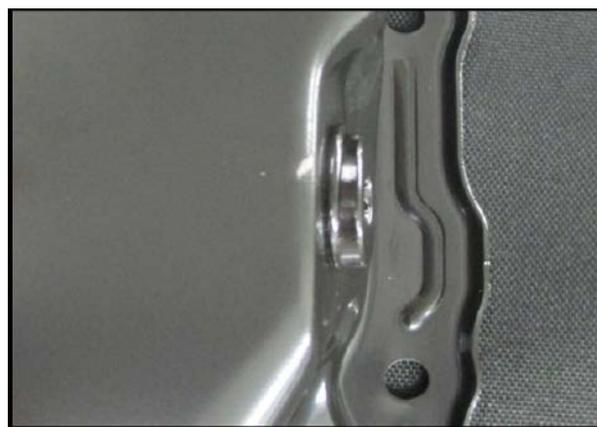
If the oil pan is flat, use drain plug and washer:
