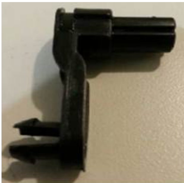
Installation of the passenger side temperature flap lever. (Black)
