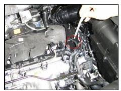
Hose not inserted into the vacuum container.
