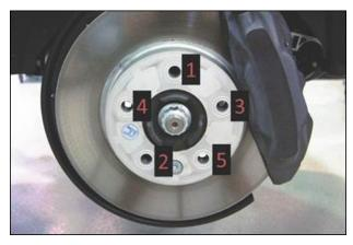
Tighten all the wheel bolts in the star pattern specified in the picture.
