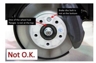
Example of improper positioning.
