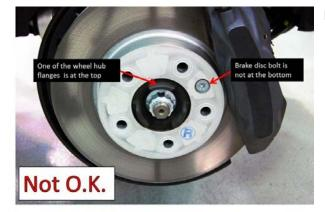
Example of improper positioning.
