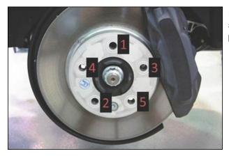
Each wheel bolt hole is assigned a number from 1 to 5. These numbers will be referenced below. (Star pattern)
