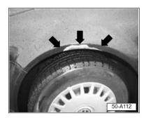
Corrosion at front fender -arrows-, as shown.
