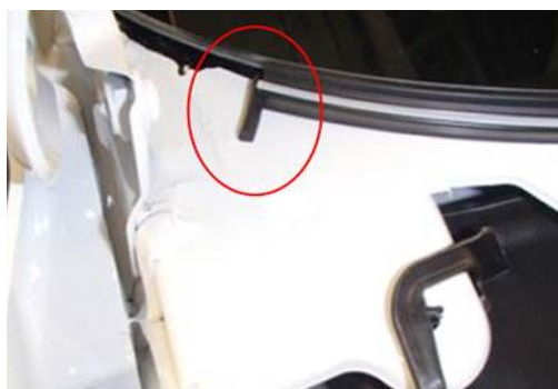
Addition of water deflector 3C0 845 237.
