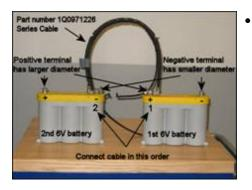
Connect cable (Part No: 1Q0971226) to inner battery terminals.
