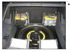
(3.2L) Test/charge AGM battery located in trunk - one 6V battery located on each side of ski chute, as shown.
