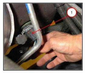
• Remove the solenoid pack connector (1) at the valve body oil pan.
