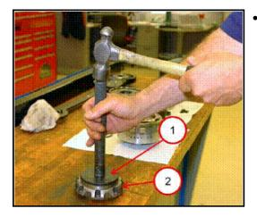
Install the new bearing <u>outer</u> race into the transfer shaft bearing retainer (2) using Bearing Race Installer 9952 and Handle C4171 (1).
