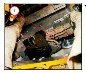
Lift up on the valve body to clear the manual valve pin (1) past the slot in the rooster comb.
