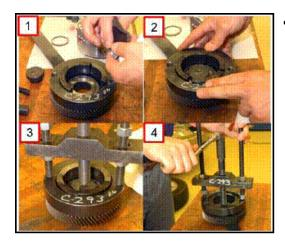
Using press puller P/N C-293-PA, Adaptors P/N 9738 and a press plug P/N 9678, remove compounder transfer gear bearing cone.
