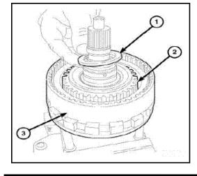
• Install thrust bearing (1) onto transfer shaft.
