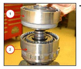
Install the direct clutch (1) onto the low clutch (2).
