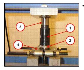
Using installer P/N 6756 and a press, install the transfer bearing Part. No. 7B0323415A onto the transfer shaft.
