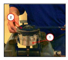
Install the transfer gear onto the transfer shaft (1) and Holder Part No. 9739 onto the transfer gear (2).
