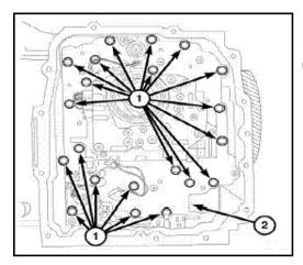
Install the twenty one valve body to case bolts and tighten to 6 Nm (50 in. lbs.).
