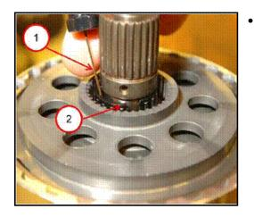
Install split bearing (2) and lock into place.
