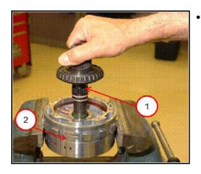
• Remove the transfer shaft (1) from the low clutch (2).
