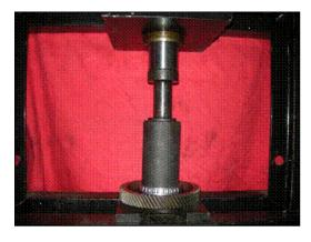
Install the transfer gear bearing cone Part No. 7B0323415A using installer Part No. 6756.
