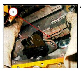
Position the valve body near the underdrive compounder oil transfer tubes and slide the valve body manual valve pin (1) into the slot in the rooster comb.
