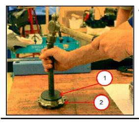
Install the new bearing <u>inner</u> race into the transfer shaft bearing retainer (2) using Bearing Race Installer 9952 and Handle C4171 (1).
