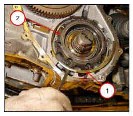
• Remove the snap ring (1) at the underdrive compounder assembly (2).
