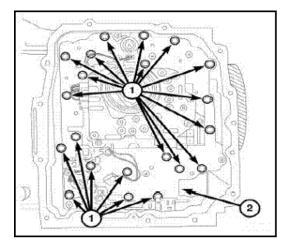
Remove the 21 valve body to case bolts (1). **One valve body bolt is hidden by the manual valve rooster comb.**
