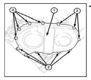
Remove transfer gear cover-to-case bolts (2) and remove cover (1).
