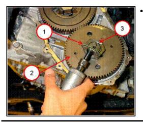
Grind the staked tabs (3) from the transfer gear (2) (underdrive coumpounder side). Take care not to damage the transfer shaft threads.
