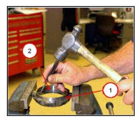
• Using a suitable tool drive the transfer shaft bearing outer race (2) from the transfer shaft bearing retainer (1).
