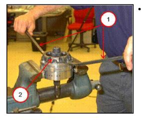
Remove remaining fasteners securing the transfer shaft bearing retainer and remove the retainer (2).
