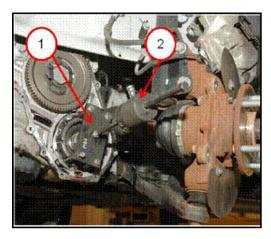
Install puller adaptor (1) P/N 9908 to the compounder bearing retainer.
