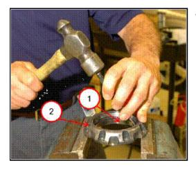
Using a suitable tool drive the transfer shaft bearing inner race (1) from the transfer shaft bearing retainer (2).
