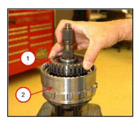
• Install overrunning clutch (1) into low clutch (2).
