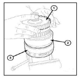
Remove the slide hammer from the adaptor P/N 9908 and clamp the adaptor into a vise to support the underdrive compounder (3) during the disassembly process.
