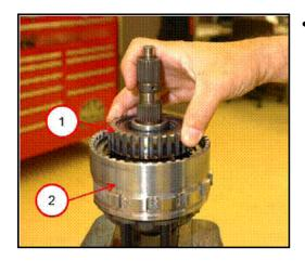
• Remove the overrunning clutch (1) from the low clutch (2).
