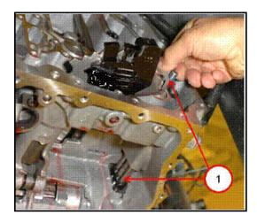
• Separate the underdrive coumpounder transfer tubes (1) from the underdrive compounder.
