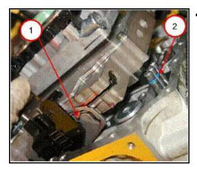
• Pull the valve body away from the underdrive compounder oil transfer tubes (2).
