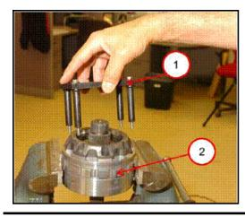
• Carefully clamp the underdrive compounder low clutch (2) into a soft jaw vise.
