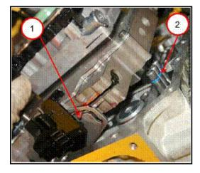
Slide the valve body onto the underdrive compounder transfer tubes (2).
