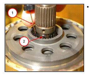
Remove the split bearing (2) using a small pick.
