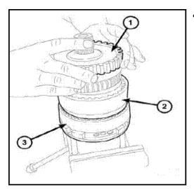
• Install the planetary gear (1) set/output hub onto the direct clutch (2).
