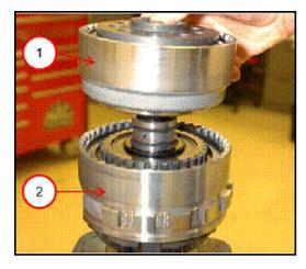
• Remove the underdrive compounder direct clutch (1) from the low clutch (2).
