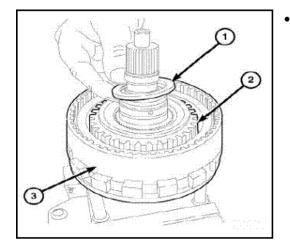
Remove the thrust bearing (1) from the transfer shaft.
