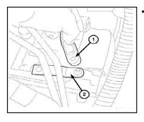
Remove shift cable (1) from manual valve lever (2).
