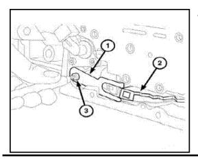
• Remove the screw (3) at the detent arm (1) and remove arm.
