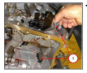
Install the underdrive compounder oil transfer tubes (1) into the underdrive compounder.
