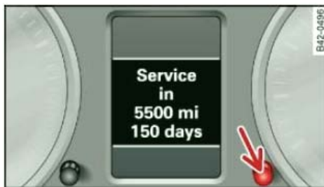
Fig. 19 Section of instrument cluster: Service interval display
