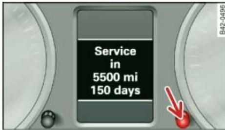
Fig. 19 Section of instrument cluster: Service interval display
