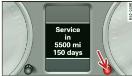
Fig. 19 Section of instrument cluster: Service interval display
