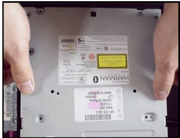
Figure 7. Pry top cover off with fingers.
