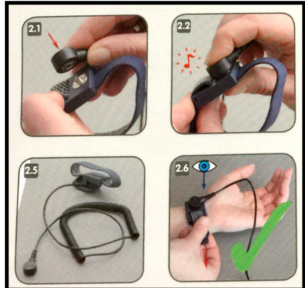
Figure 3. VAS6613 ESD work surface grounding wrist strap.
