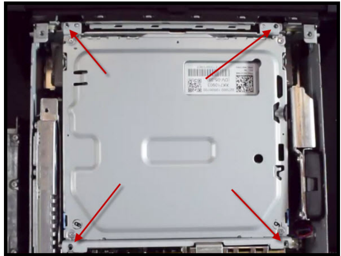
Figure 11. CD drive mounting points are now free.
