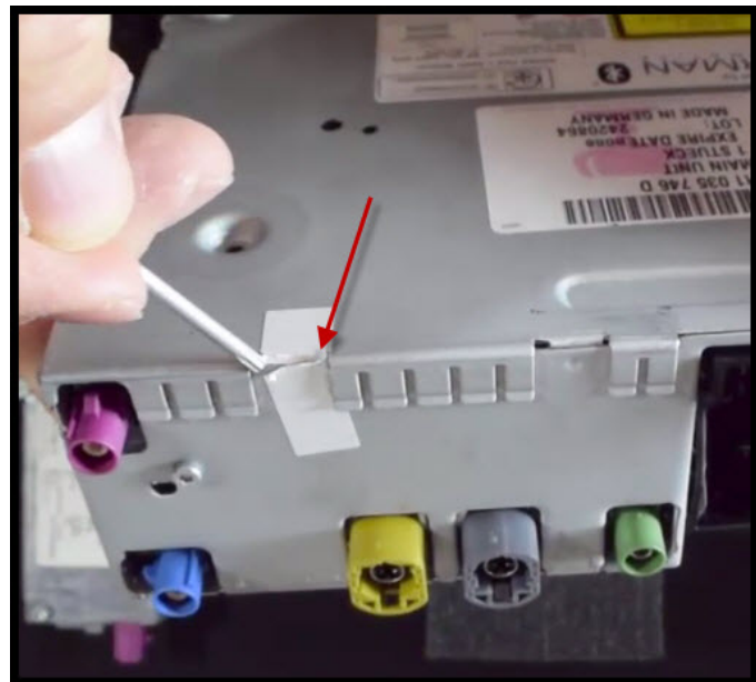
Figure 7. Break the white warranty seal.
