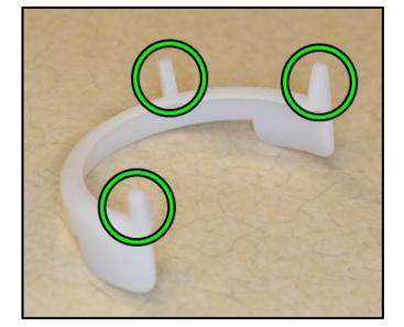
The retaining ring is installed into the filler neck with the alignment pins <circles> facing toward the fuel tank.
