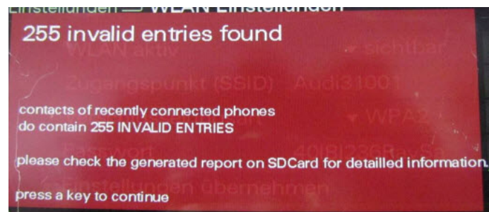
Figure 5. Specific issues were detected with the phonebook contact entries
