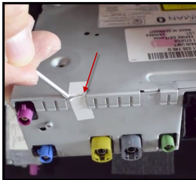
Figure 7. Break the white warranty seal.
