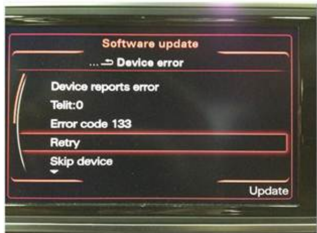
Figure 7. A device requiring a 'Skip device' selection.
