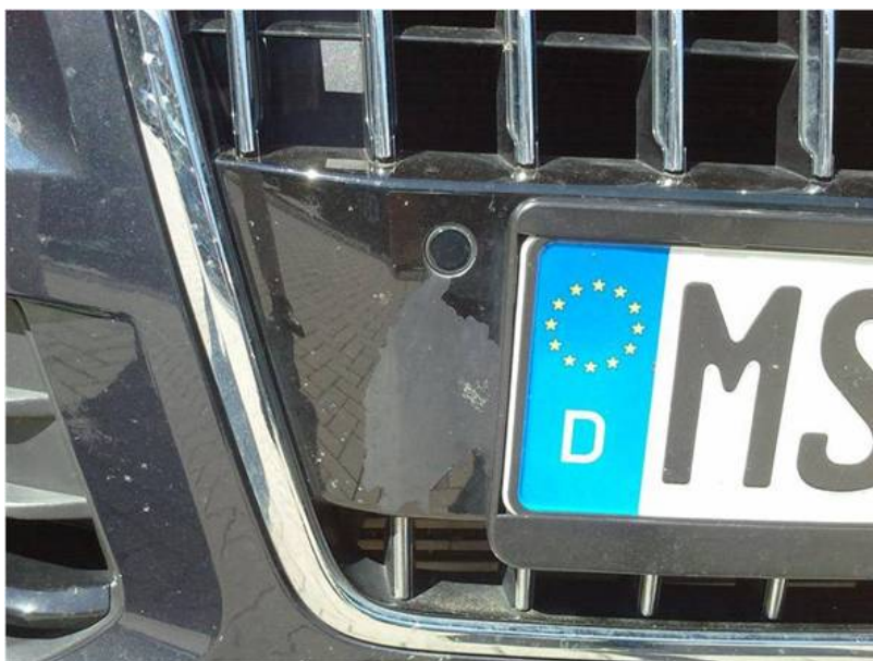
Figure 1. Example of flaked-off paint.
