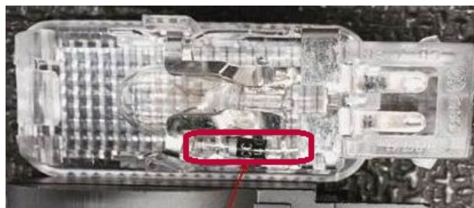
Figure 1. Trunk light 3B0947415B with protective diode. The protective diode is circled.
