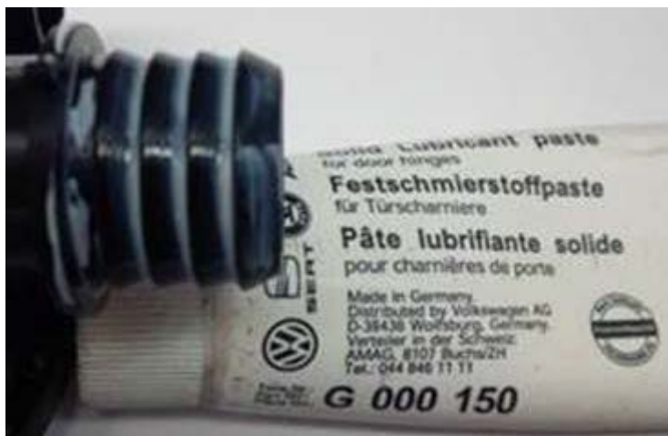
Figure 5. Grease film on outer surface of grommet.
