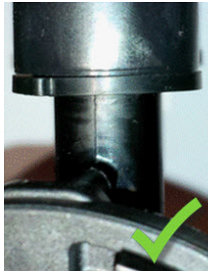
Figure 6. Correctly-installed sensor and grommet.
