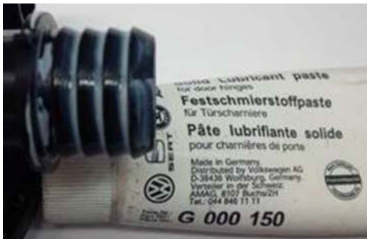
Figure 5. Grease film on outer surface of grommet.
