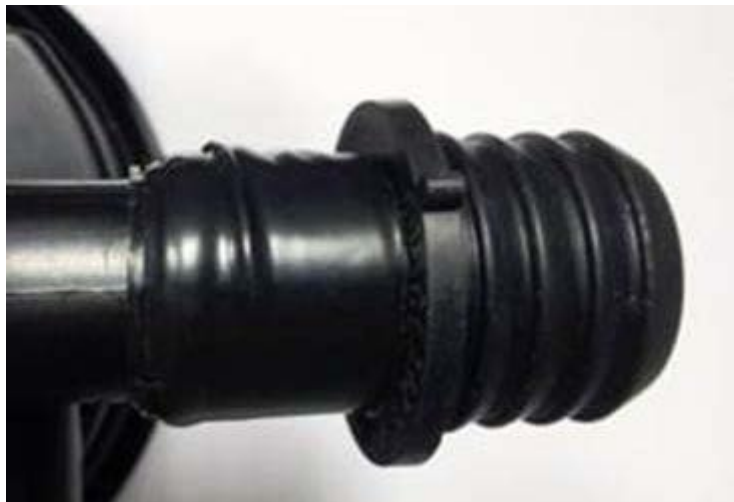
Figure 4. Vinyl layer supporting grommet.
