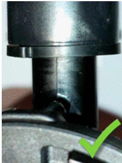
Figure 6. Correctly-installed sensor and grommet.
