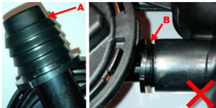
Figure 7. Plastic port extending past the grommet (A) causing installation issues (B).
