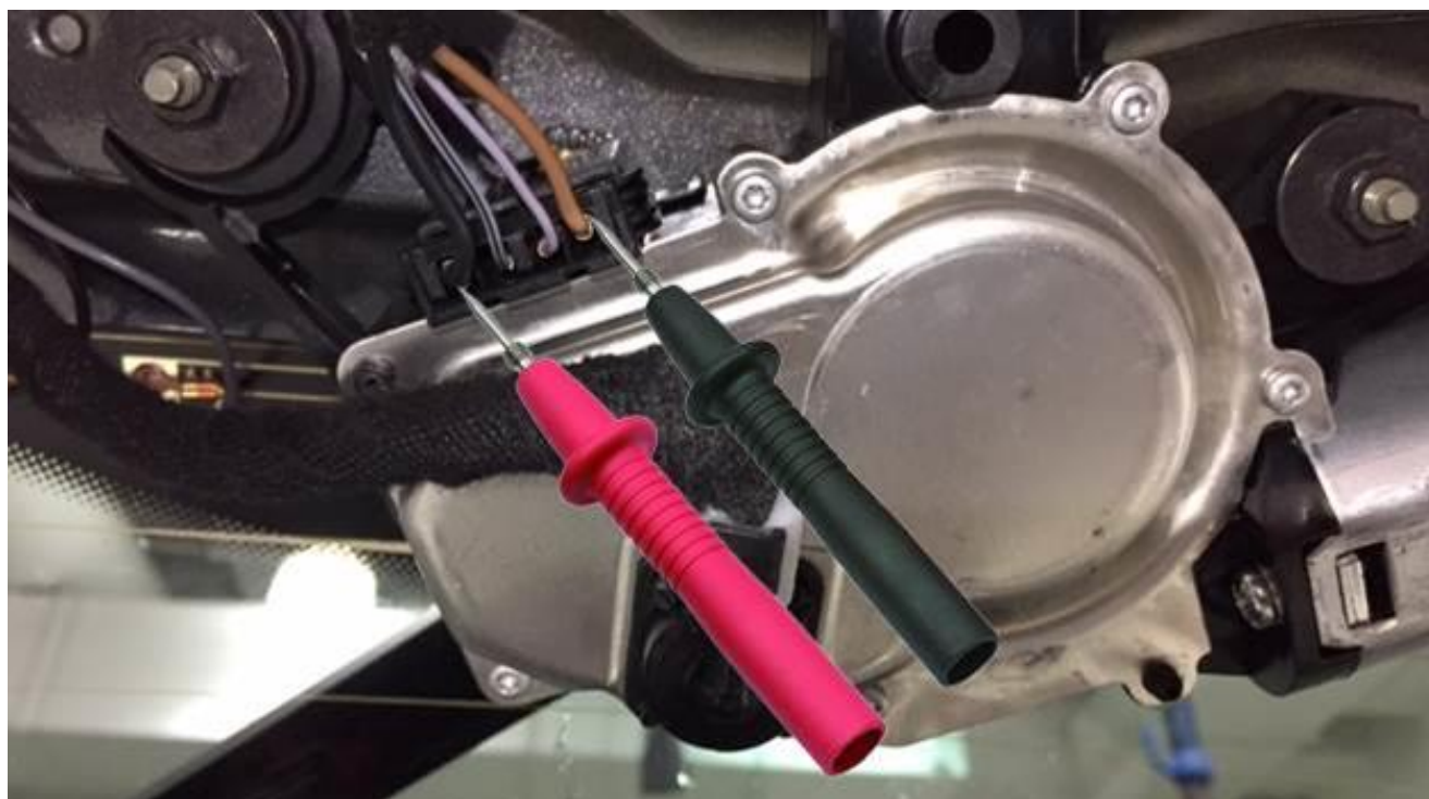
Figure 4. Check voltage at pin 1 and pin 4.
