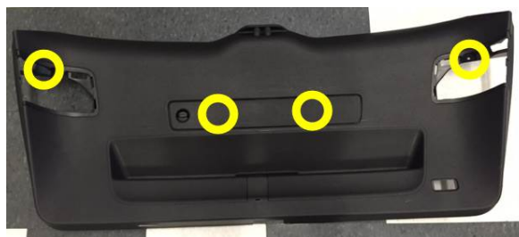
Figure 1. Screw location on lower tailgate trim.
