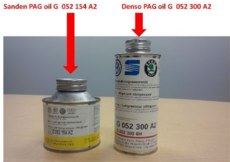
Figure 3: Compressor manufacturer specific PAG oils.
