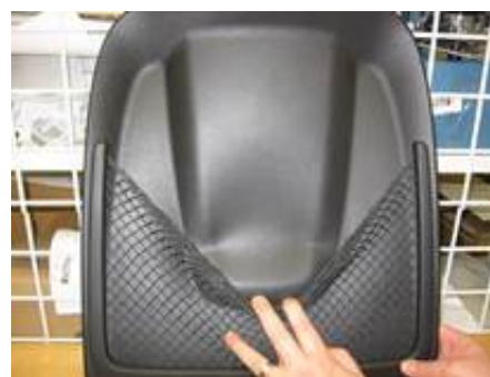
Figure 1. Damaged front seatback panel.
